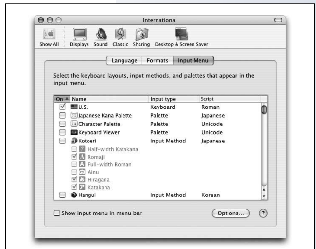
Figure 3-16. The Input Menu pane of International settings allows you to select keyboard layouts and palettes that help you build rich, multi-language Unicode files.
